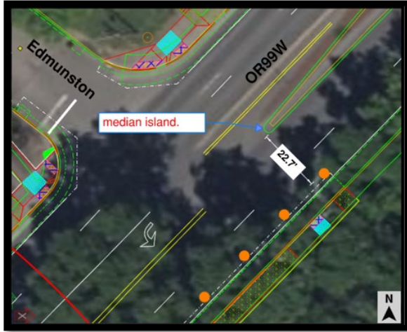
Figure 4: Available horizontal clearance on OR99W at Edmunston Street during non-work hours
