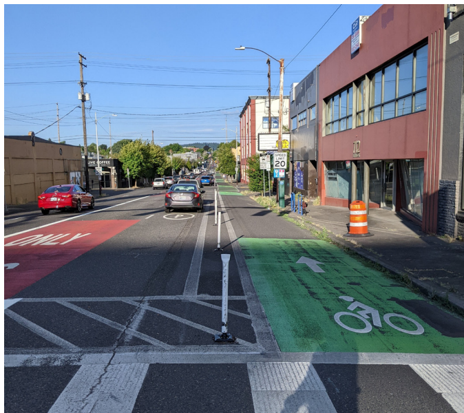
Parking protected bike lane and bus only Rose Lane on SE Hawthorne Boulevard at 7th Avenue .
