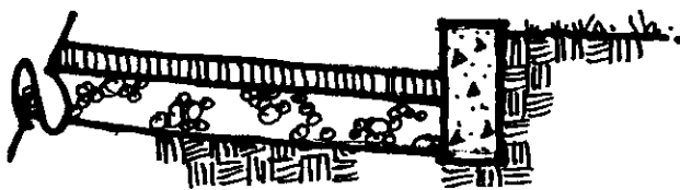
Figure 5.8- Standard Curb Section
