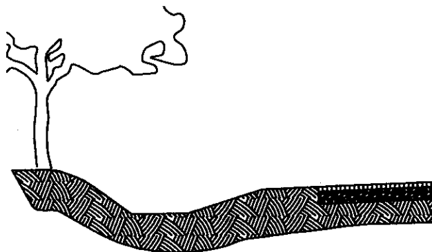
Figure 4.15 - Swale for Stormwater Treatment
