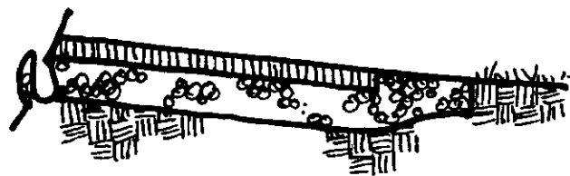
Figure 5.10- Section with No Curb
