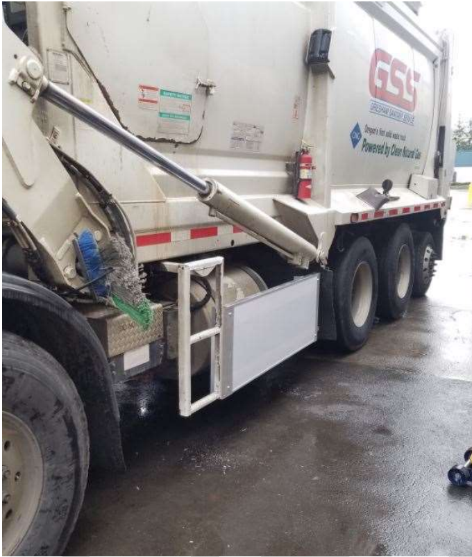
Left: front-load truck with panel side guard. Below: front-load truck with panel side guards and warning sticker. Bottom of page: rear-load truck with rail side guards.
