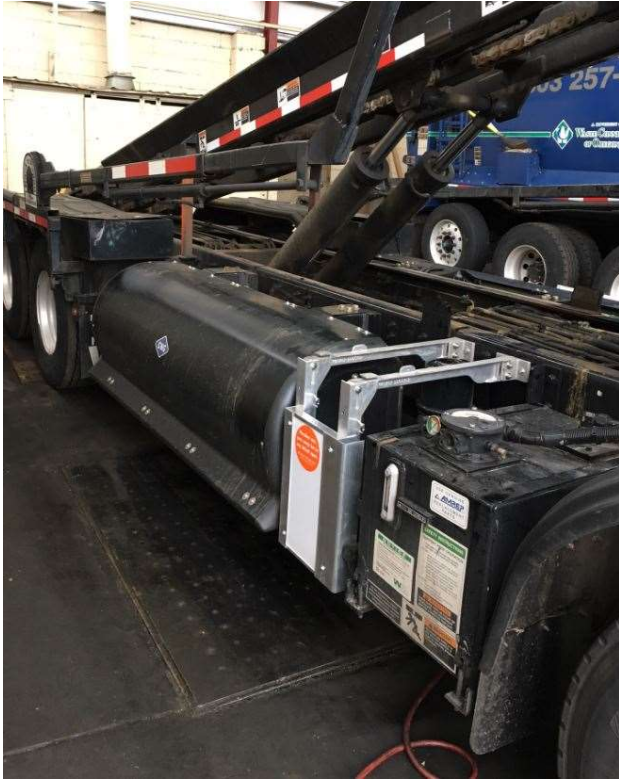
Left: drop-box truck with small openings and panel side guard and warning sticker. Below: drop-box truck with rail side guards. Bottom of page: side-load truck with panel guards and warning stickers.
