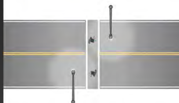
Figure 12. Drawing. New design for midblock crosswalk lighting layout.
