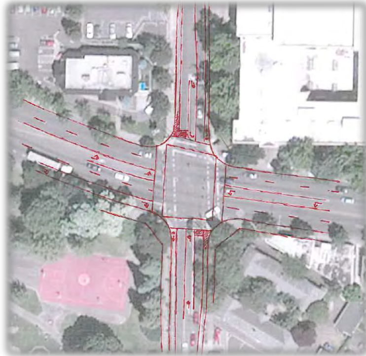
Exhibit 41 Concept to Accommodate Wider Bike Lanes on Both Sides of 26 th Avenue
