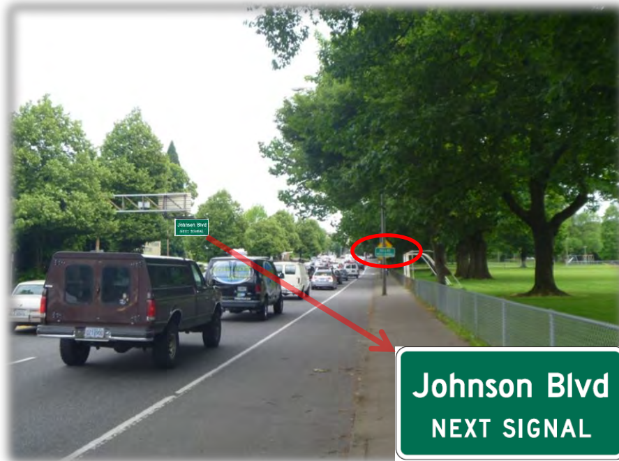
Exhibit 16 Example of Using Cantilever for Next Signal Sign at Eastbound Approach to 26 th Avenue
