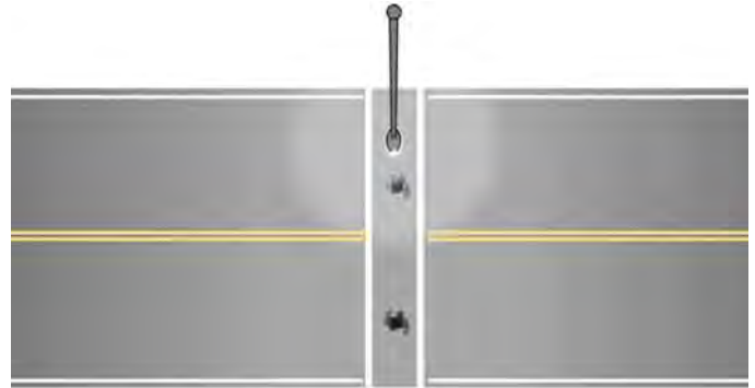
Figure 11. Drawing. Traditional midblock crosswalk lighting layout.
