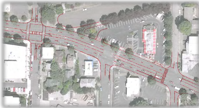
Exhibit 56 28 th Ave Traffic Signal Allowing Pedestrian and Bike Crossings and Right-turns Only
