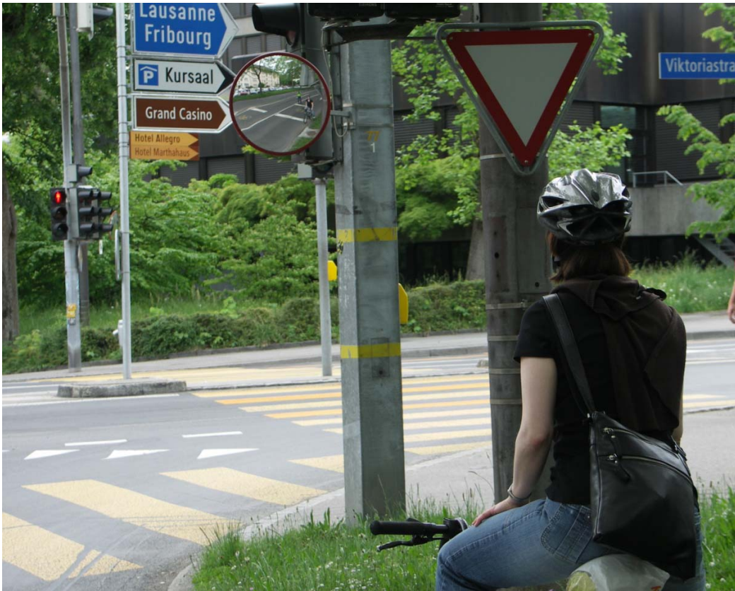
Figure 3. Convex Mirrors Improve Bicyclist Visibility for Drivers of Large or High-Profile Vehicles (Bern, Switzerland)
