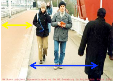
Willemsbrug Rotterdam, Netherlands 6' sidewalks (2) 6' bike lanes (2) Total: 24'
